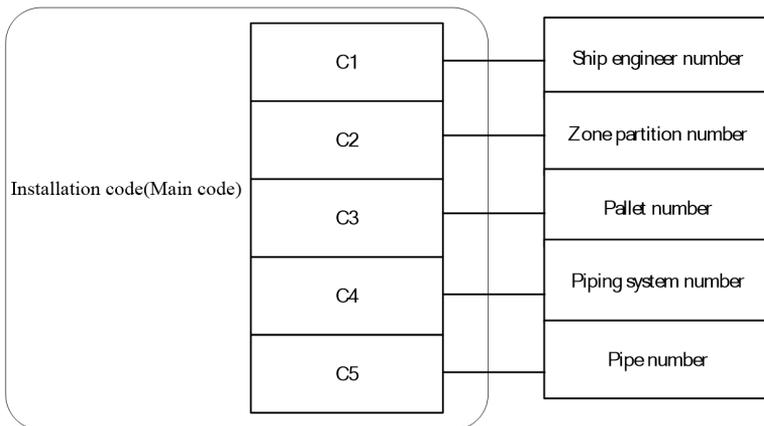
Fig. 3. Tube-oriented structure for the installation
